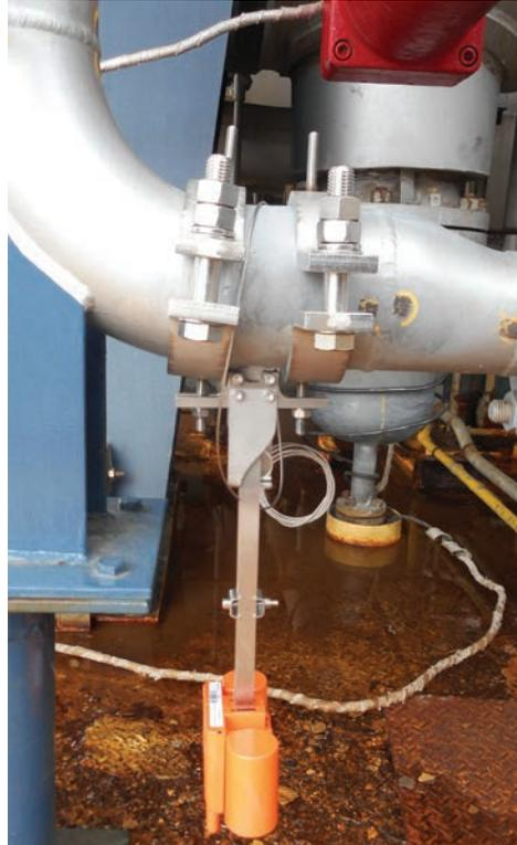
**FIGURE 5.** Ultrasonic corrosion sensors can be permanently installed on a pipe line
