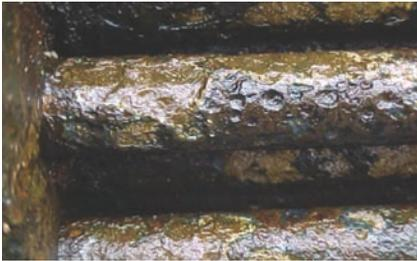
**FIGURE 4.** Corrosion in crude overhead
