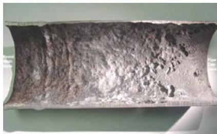
**FIGURE 2.** High TAN crudes cause naphthenic acid corrosion
